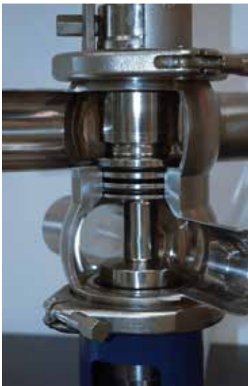
Shaft and body from solid bar
