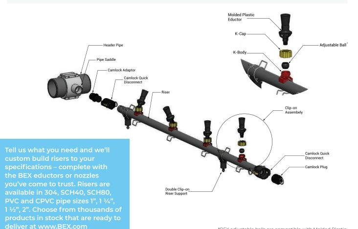
\*BEX adjustable balls are compatible with Molded Plastic Models T00MP, T0MP, and all Mini Plastic Models.
